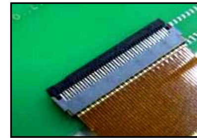
FH35C Series Pitch: 0.3 mm Height: 0.9 mm Back Flip (Top & Bottom Contact)
